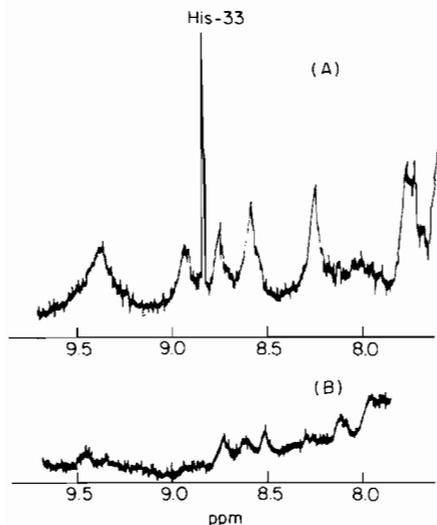
Fig. 1. Proton NMR spectra (Bruker WH500) of (a) cyt *c* and (b) *cis*-[Ru(en)<sub>2</sub>(OH)](His-33)cyt *c* in the region of imidazole <sup>1</sup>H resonances (D<sub>2</sub>O/DCl, pH 5.5; internal DSS).
